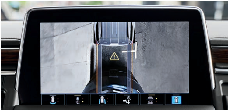
Rear Top-Down View Shows the clearance between the rear of the vehicle and nearby objects.
